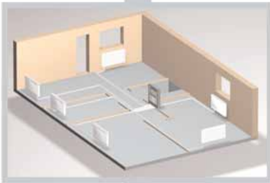
Example of a homerun distribution system
