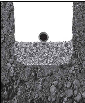
Trench in bad soil
