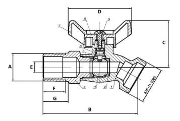
This approved Webstone valve is designed for attachment to outdoor faucets and for use with water. Threaded ends comply with ASME B1.20.1.
