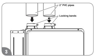
Insert a 2" PVC pipes slowly into an air intake connector and a flue connector located on top of the water heater until they stop. **DO NOT** use cement. Tighten 2 locking bands to secure 2" PVC pipes.
