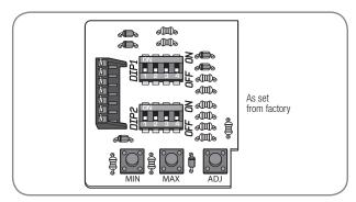
A-1 setting is default and factory setting. All dip switches are off.
