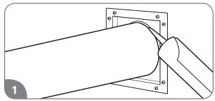
Apply silicone sealant or silicone/latex caulk to seal the vent pipe to the vent coupling to permit field disassembly for annual inspection and cleaning. Completely seal where it passes through the wall plate and where it is attached to the structure.
