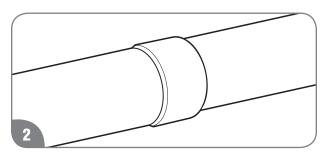
Attach the female end of the next vent pipe section to the male end of the 2-in./3-in. (5.1-cm/7.6-cm) vent pipe. See "Cementing Joints" on this Use and Care Manual.
