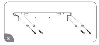
Attach the mounting bracket to the wall and secure it by 4 screws and washers. Make sure it is level and that it can support the weight of the water heater.
