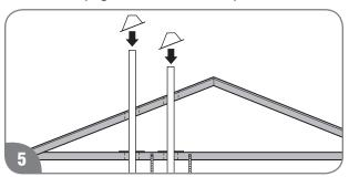
Install adequate flashing where the vent pipe passes through the roof.
