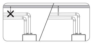
The unit may be vented horizontally through a wall or vertically through the roof. Pipe runs must be adequately supported along both vertical and horizontal runs. Maximum unsupported span is recommended to be no more than 4 feet (1.2 m). It is imperative that the first hanger be located on the horizontal runs immediately adjacent to the first 90-degree elbow from the vertical rise. Only use support isolation hanging bands. DO NOT use wire to support pipe runs.
