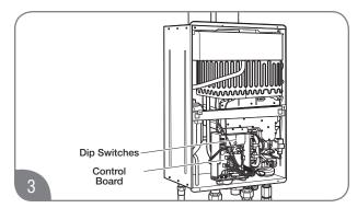
Find DIP Switch 2 located in the top-right portion of the control board. The switch labeled "DIP 2" is the bottom switch.
