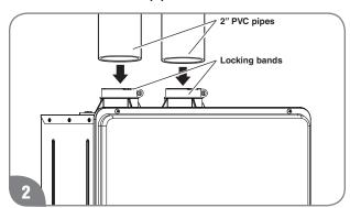
Insert a 2" PVC pipes slowly into an air intake connector and a flue connector located on top of the water heater until they stop. Tighten 2 locking bands to secure 2" PVC pipes.
