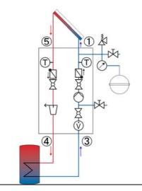
5. Connect the solar station to the system by means of pipes
