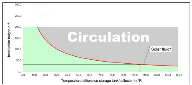
• The installation height between the collector and the storage tank is ~33 ft (10 m).
