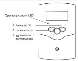
The controller is operated via the 3 push buttons below the display.
