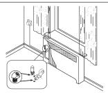
Available for mounting the 1PS assembly onto convectors are 1/8" 45° street elbows, part number 013L8300. When ordering these elbows two pieces are needed per convector.
