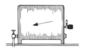
Make sure that free-standing radiators or cast iron convectors are properly pitched and that hand valves are FULLY open.
