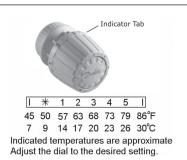
The user can easily set room temperature by turning the dial clockwise or counterclockwise. The diagram to the left shows the approximate relationship between dial scale numbers and room temperature.
