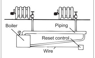
Boiler/Steam supply must be cycled by a reset control or room thermostat and must not run at constant pressure (which would prevent air from entering back into the system).
