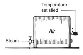
To aid in preventing overheating of rooms that are temperature satisfied, boiler steam pressure must be kept low, recommended normally at or below 2 psig. Otherwise air will be compressed in the radiator, allowing steam to enter when not required.
