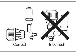
The operator with valve-mounted dial and sensor must be mounted horizontally.
