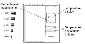
\* The thermostat displays the percentage of heating time required to maintain the desired temperature. For example, \$\$ is displayed when heating is activated 40 percent of the time.
