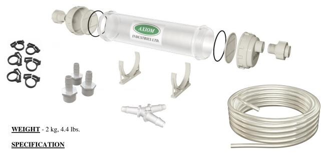
The condensate neutralization capsule shall be AXIOM INDUSTRIES LTD. model NC-1. System shall include 1 litre (0.26 U.S. gallon) transparent capsule made from corrosion resistant materials with two 3" fill/access openings, 3" inlet and outlet screen, 3/4"-14NPT threaded inlet, 3/4"-14NPT threaded outlet, two 3/4" MNPT x 3/4" FNPT unions, three 3/4" NPT to 1/2" hose barb fittings, 1/2" barbed Y fitting, six hose clamps, 10 ft of 1/2" ID vinyl tubing, two base/wall mounting clamps.
