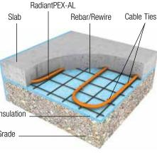
Pour concrete over for heating or snow melting
