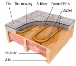
Install in a thin concrete, gypsum or self-leveling floor.
