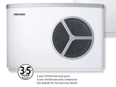
The integral anti-vibration mount enables the heat pump to be connected directly to the heating system, with a pivoting electrical connection panel for easier installation. The condensate pan is easily reached through a cleaning aperture on the back of the casing. The enamelled, corrosion-protected metal casing in alpine white is made from hot-dip galvanized, powder coated sheet steel. Fan grill, recessed grips and top cover are made from weatherproof, UV-resistant plastic in aluminum white.
