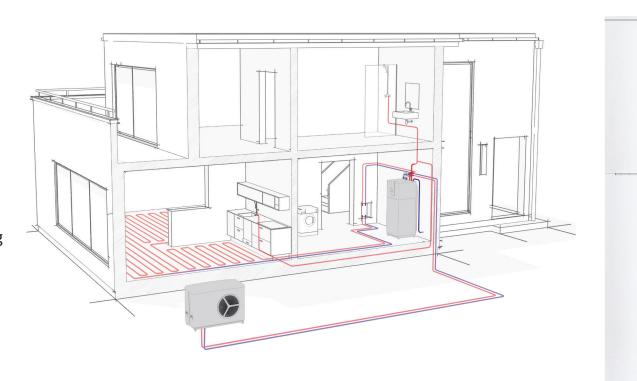
Flow temperatures of up to 149°F/65°C are achieved even at low outside air temperatures due to a combined enhanced vapor injection/enhanced saturated vapor injection that cools the scroll compressor. The high flow temperature makes the WPL capable of use in modernization projects that may need a high flow temperature, as well as in construction, new or old, designed for lower flow temperatures.
