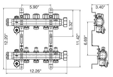
\* When extending the manifold, Viega requires using thread sealant paste on the 1" NPT manifold end connection.
