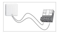
If an optional indoor sensor (Part Number 16016) is used, connect the two wires from the sensor to the Com and Indr terminals (11 and 13) (Part Number 16016).
