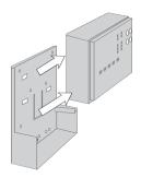
5. The control lifts up and away from the base, which is ready for mounting.
