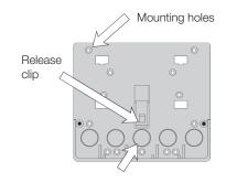
Remove the control from its base by pressing down on the release clip in the wiring chamber and sliding the control upward. The base may then be mounted by screwing it to a wall or mounting board (screws not included).
