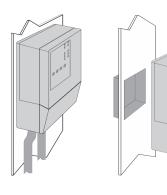
6. Wiring can enter from bottom or back of enclosure. Knockouts allow wiring to be run in conduit.
