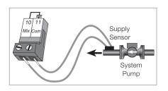
Connect the two wires from the Supply Sensor to the Com and Mix terminals (10 and 11). The Supply Sensor is used by the Basic Heating Control to measure the supply water temperature downstream of the diverting or mixing valve.
