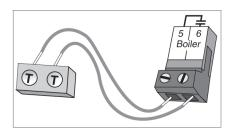
Do not apply power to these terminals as this will damage the control.
