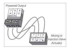
Terminals 7, 8, and 9 are powered with 24V AC from the control. There is no need to provide a separate 24V AC power source for the valve actuator.
