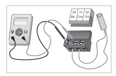
In order to test the sensors, the actual temperature at each sensor location must be measured. A good quality digital thermometer with a surface temperature probe is recommended for ease of use and accuracy. Where a digital thermometer is not available, a spare sensor can be strapped alongside the one to be tested and the readings compared. Test the sensors according to the instructions (see "4.7 Testing the Control" on page 26
