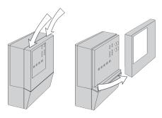
1. Press down at grips on top of cover, then pull out and down to release cover.
