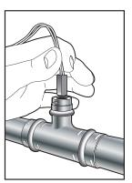
The Supply Sensor should be placed downstream of a circulator pump or after an elbow or similar fitting. This is especially important if large diameter pipes are used, as the thermal stratification within the pipe can result in erroneous sensor readings. Proper sensor location requires that the fluid is thoroughly mixed within the pipe before it reaches the sensor. When using the Supply Sensor with a Mixing Station, insert the sensor into the immersion well, see image to the left.
