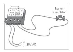
The Sys Pmp output terminal (3) on the Basic Heating Control is a powered output. When the relay in the Basic Heating Control closes, 120V AC is provided to the Sys Pmp terminal (3) from the Power L terminal (1). To operate the system circulator, connect one side of the system circulator circuit to terminal (3) and the second side of the circulator circuit to the neutral (N) terminal (4).
