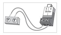
If the boiler is connected to the boiler terminals (5 and 6), make sure power to the boiler circuit is off and install a jumper between the terminals. When the boiler circuit is powered up, the boiler should fire. If the boiler does not turn on, refer to any installation or troubleshooting information supplied with the boiler. (The boiler may have a flow switch that prevents firing until the boiler pump is running.) If the boiler operates properly, disconnect the power and remove the jumper.
