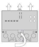
4. Press release clip on base and slide control upward.
